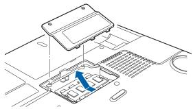
Figure 4-11. Opening the Memory Upgrade Compartment
